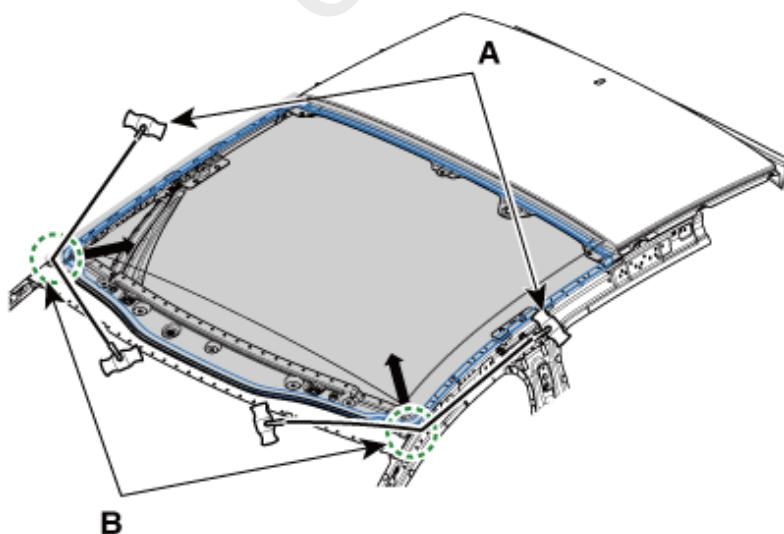
12. Push wire (A) from the outside of the body toward the face of edge (B) in the direction of the arrow.
