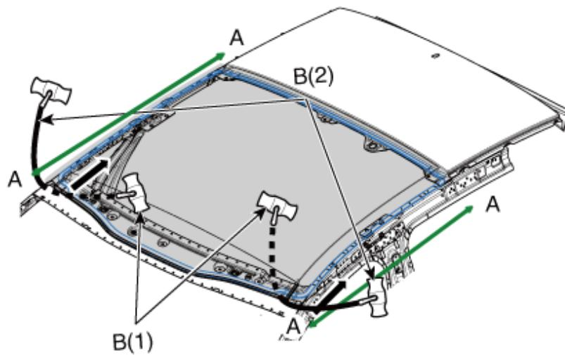
16. Pull the square wire (B) to the left and right, then apply a force in the direction of the arrow to cut off the residual sealant on rear section (A-A).
