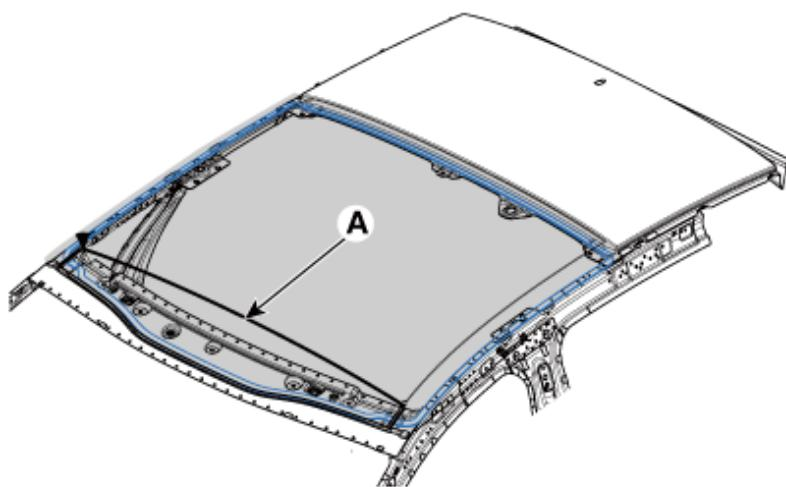
19. Check step and gap before front glass (A) is fully mounted.
