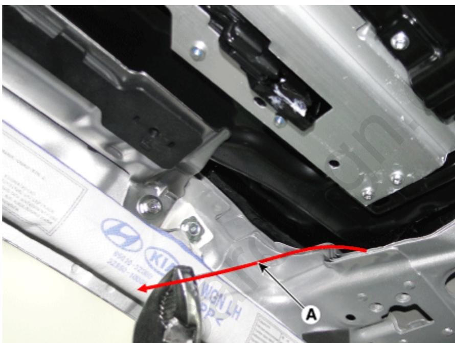
14. Pull the square wire (B) to the left and right, then apply a force in the direction of the arrow to cut off the residual sealant on front section (A-A).
