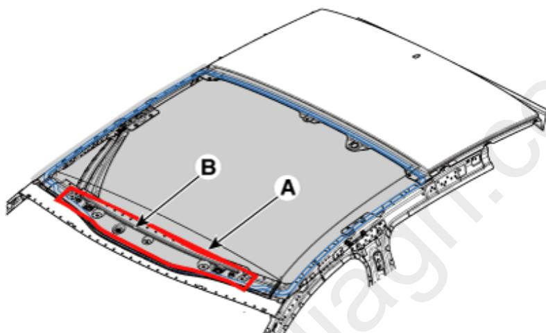
18. Install the front glass (A) loosely on the body panel.
