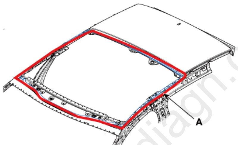
2. If panorama sunroof assembly (A) is reused, use a blade to remove residual sealant (B) around the body panel.
