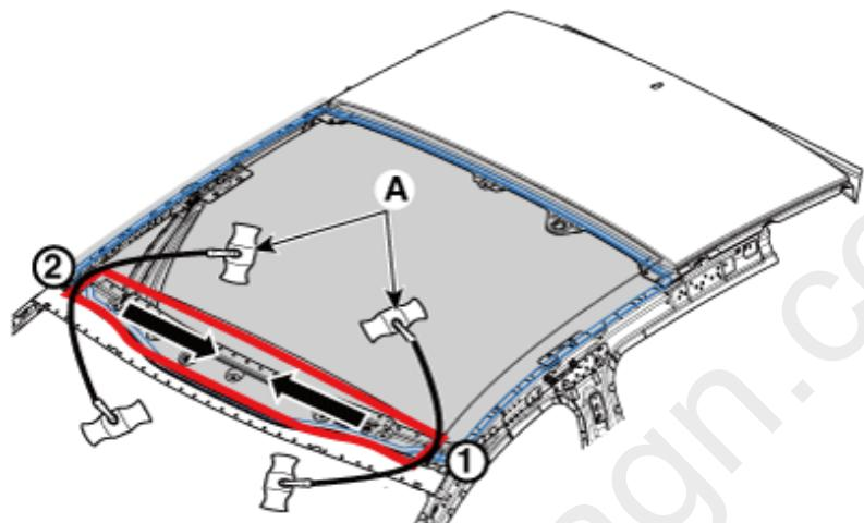
8. Remove the front glass (A) carefully without damaging it.
