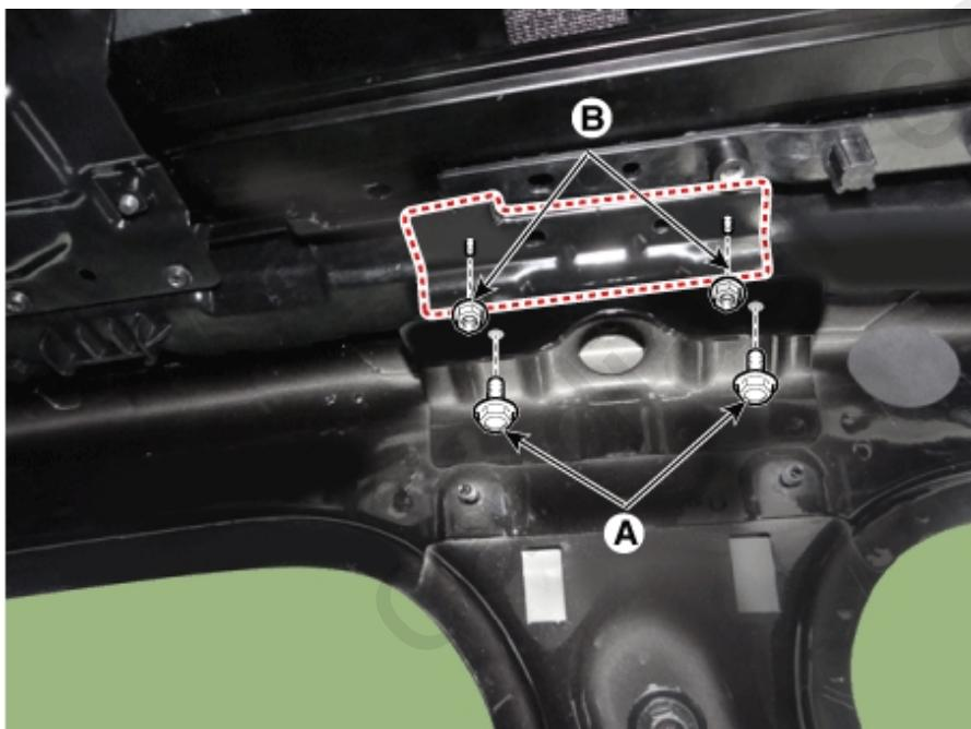
10. Install the assist handle bracket (A).
