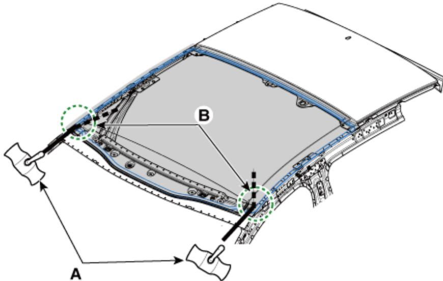
13. Pull the wire lead (A) inward when it is visible inside the body.
