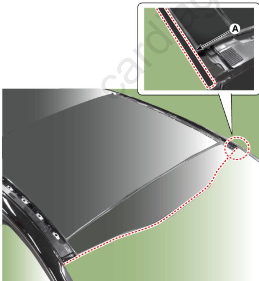
7. Pull the square wire (A) to the left and right, then apply a force in the direction of the arrow to cut off the residual sealant.
