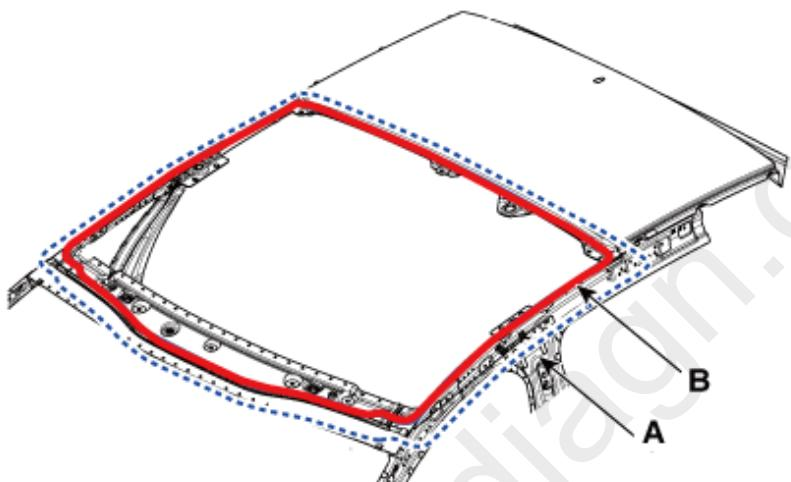
5. Align with centering device hole (A) of the body, and carefully mount the panorama sunroof on the body panel.
