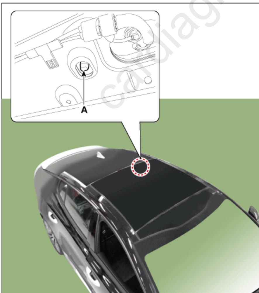
6. Check step and gap before fully mounting panorama sunroof assembly (A).
